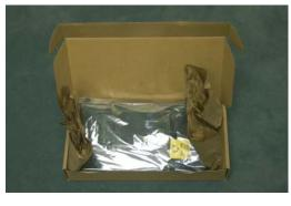
CIRCUIT BOARD SAFELY AND SECURELY PACKAGED IN STATIC SHIELD BAG WITH PAPER DUNNAGE TO CUSHION AND SECURE UNIT WHILE IN TRANSIT.
