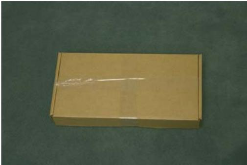
CIRCUIT BOARD SECURELY ENCLOSED IN SERVICEABLE BOX. BOX TAPED CLOSED BOTH DIRECTIONS.
