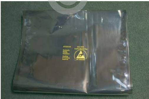
USE STATIC SHIELD BAGS TO STORE, TRANSPORT AND SHIP CIRCUIT BOARDS.
