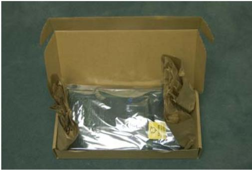
CIRCUIT BOARD SAFELY AND SECURELY PACKAGED IN STATIC SHIELD BAG WITH PAPER DUNNAGE TO CUSHION AND SECURE UNIT WHILE IN TRANSIT.
