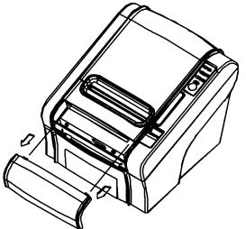
3. Turn screw with drivers to a direction until paper is released from the cutter.
