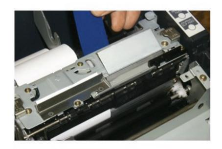
Gently slide your handy paper jam remover through the paper route. Be careful not to force the handy paper jam remover as it will damage the delicate paper press plate.
