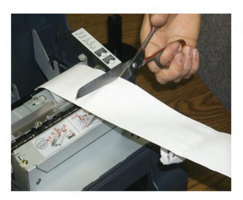
When installing a new paper roll, always cut approximately 1 foot of paper from the leading edge of the paper.
