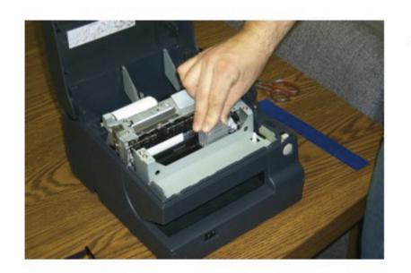
Gently slide the print head to the side furthest from the paper printing path with a paper jam.
