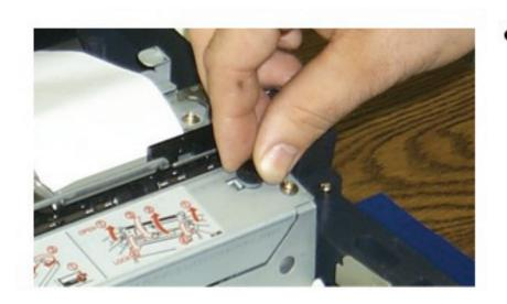
Loosen the set screw and carefully remove the coin cover when cleaning the printer or repairing a paper jam.
