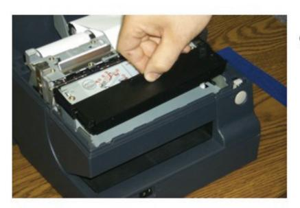
Carefully remove the printer ribbon before changing paper or repairing a paper jam.
