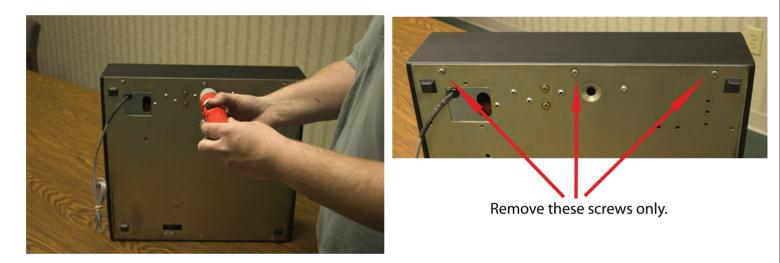
2. Remove the three screws located across the top back rear bottom edge of the cash drawer.
