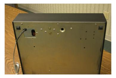
1. Disconnect the cash drawer from its power and communication source. Place cash drawer face down in order to access three screws on bottom rear back of drawer.
